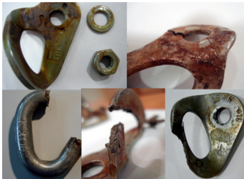
Anchors subjected to corrosion in a marine environment. Photo: Petzl
